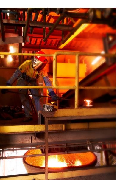
The HIsarna process can be used to create slags rich in Ti, V and/or P depending on the raw materials selection.
